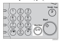
The machine will stop storing the original and the data will not be sent.
