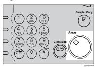
The machine starts calling the destinations. After scanning, the machine will return to standby mode.
